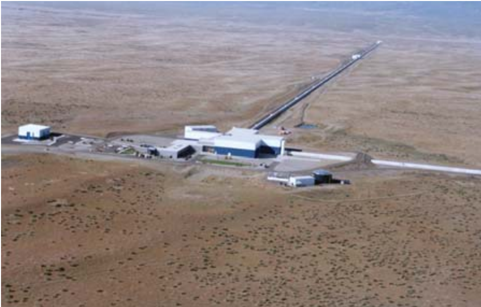
LIGO INTERFEROMETERS, such as this one at the Hanford Observatory in Richland, Wash., should be able to detect the gravitational radiation of colliding neutron stars from a distance of billions of light-years. If these signals arrive at the same time as gamma-ray bursts, a decades-old mystery may be solved.
